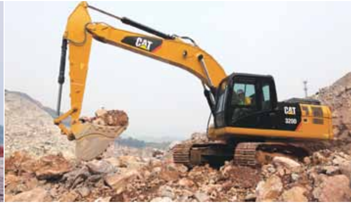
Cat 320D hydraulic excavator.
