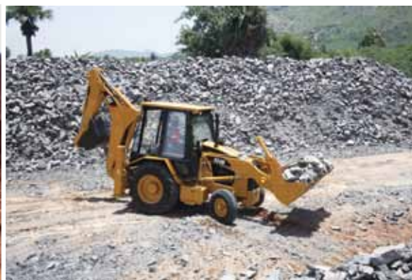
Cat 424B backhoe loader.
