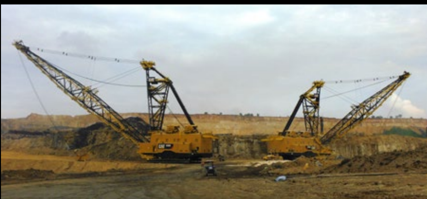
Ultra large walking draglines of 4,500 tonne with bucket capacity of 60-65 tonne.
